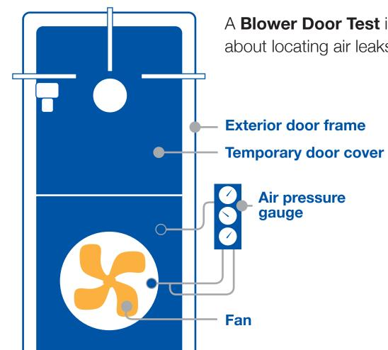
A Blower Door Test is conducted to pinpoint where buildings are losing energy. It's all about locating air leaks and ultimately making new and old buildings more energy-efficient.
